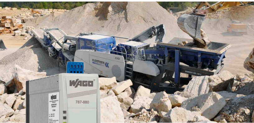
Capacitive buffer modules maintain power supply within the control cabinet, even during a temporary voltage drop when starting the motor of an impact crusher.
